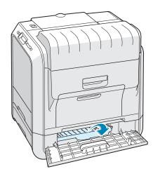
**5** Pull the jammed paper out in the direction shown. To avoid the paper tearing, pull it out gently and slowly.
